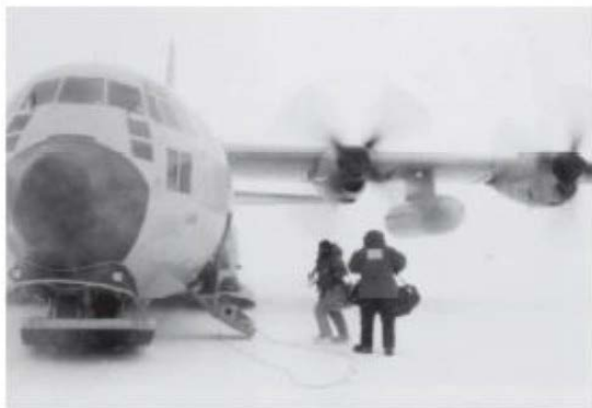
An Air Force LC-130, equipped with skis for landing, transports scientists and workers to Antarctica and back.
